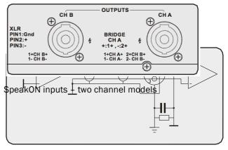
Connect the + and - loudspeaker cables as shown in the illustrations below.
