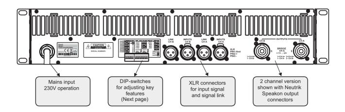
Rear view of two-channel model fitted with SpeakON connectors
