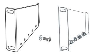
Alternative 1: Use screw and washer for fixed installation.
