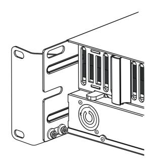
Alternative 2: Use two screws and washer for fixed installation.
