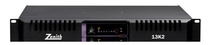
The amplifier's front panel presents the performance and fault condition indicators, power and remote switches, and a removable dust-filter cover. Level potentiometers provide individual attenuation for the amplifier channels. Range is 0dB to - infinity. (The 12 o'clock position indicates -10dB attenuation.)
