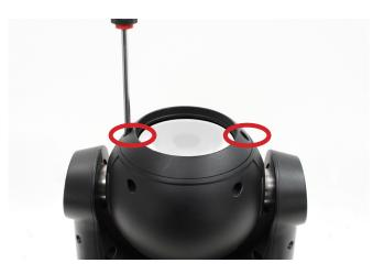
5) Tighten the screws until the plastic cover is secure.
