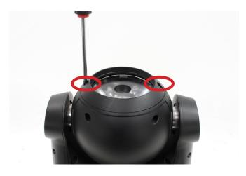
1) Place the fixture on a flat surface and unscrew the plastic cover.
