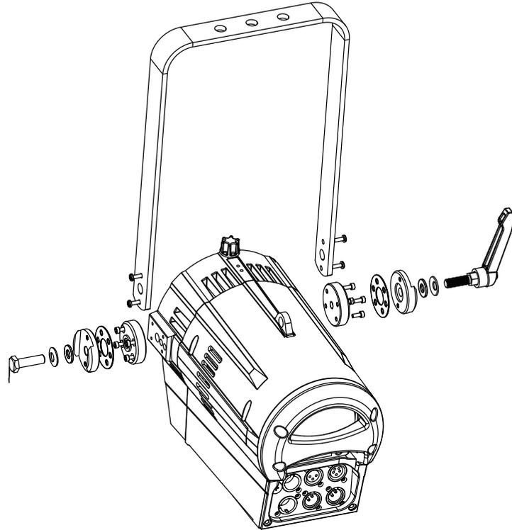
Remove the original bracket from the fixture.
