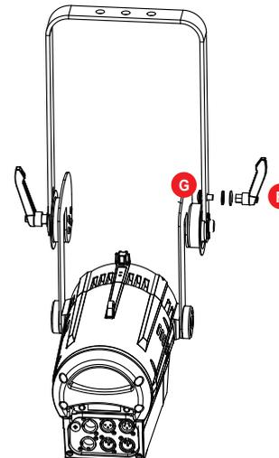
Install the M8 tightening handle onto the bracket.
