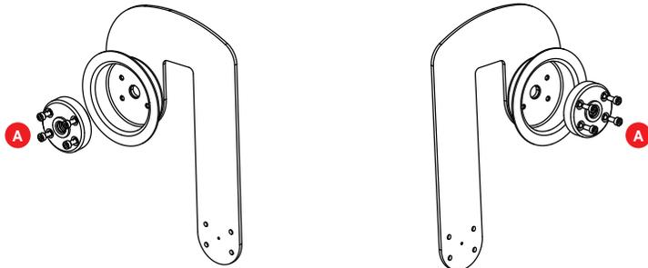
Install the positioning plate on the balance device (left and right).
