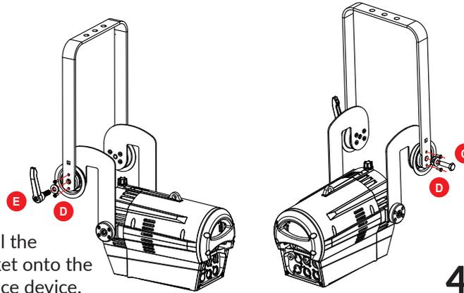
Install the bracket onto the balance device.
