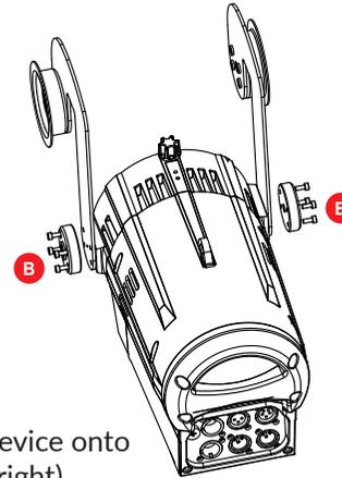
Install the balance device onto the fixture (left and right).
