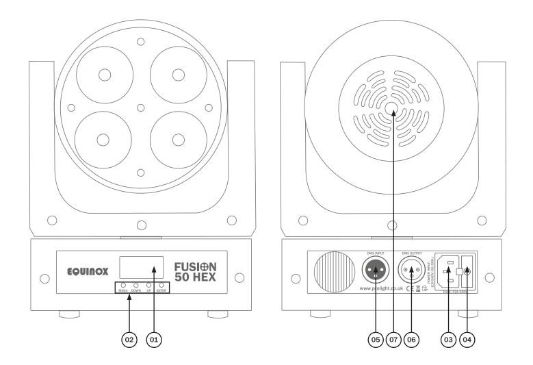
01 - LED display 02 - Function buttons 03 - IEC power input 04 - Fuse F3A 250V 05 - 3-Pin DMX input 06 - 3-Pin DMX output
