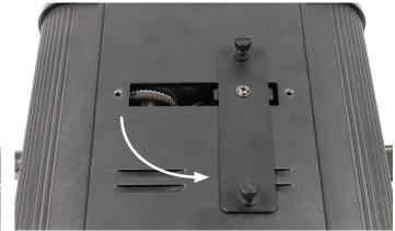
Users may change the gobos supplied for a custom design of their own. Custom gobos can be made of metal, or glass. The image size for custom gobos should be no greater than 35mmØ and the overall size of the gobo should be 44mmØ.
