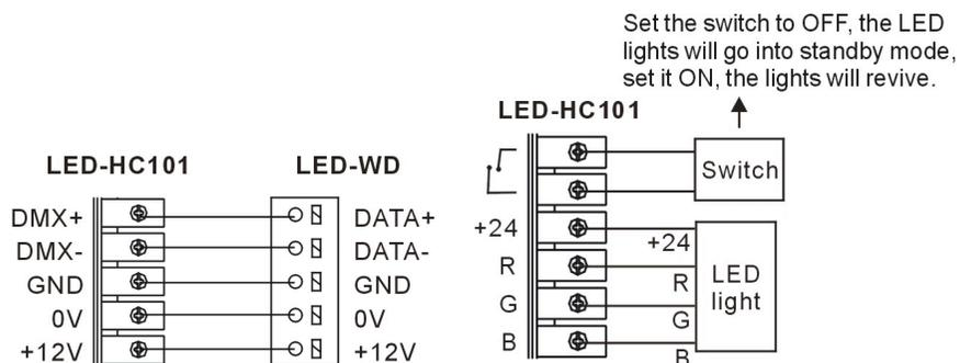
**CAUTIONS :** the LED controller total output power consumption is 100 watt.
