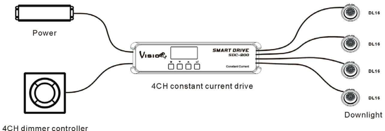
Use SDC-200 connect to four DL-16, each DL-16 unit the current is 600mA,
