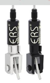
Fork head and folding spring bolt Item-No: 010-313-4040-1003 Diameter: 20mm Length: 97mm Fork size: 10mm Fork width: 20mm Spring loaded bolt: 10mm Weight: approx. 190 Gramm Color surface fork head: silver
