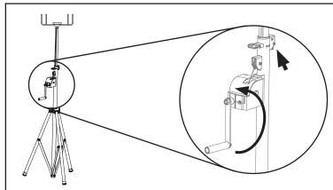
2) Press and hold the safety catch, then keeping fingers, loose clothing, and hair etc. away from the moving parts, gradually lower the system by turning the winch handle ant-clockwise.
