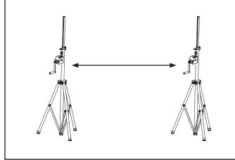
2) Fix the truss adaptor onto the top of each winch stand using the M10 bolt supplied.
