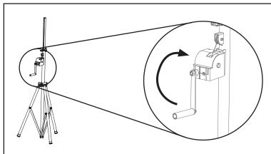
8) Raise the system to the desired height by turning the winch stand handle clockwise.
