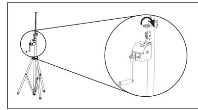
9) Tighten the locking bolts above the main winch mechanism to prevent any unwanted movement.
