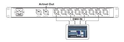
You can set any of the DMX port 1-4 as Input status. Then only the principle universal is available. It can be set within the range 0.0 - F.F. As the DMX port has been set as Input status, then the Mode only can be set as normal or backup.
