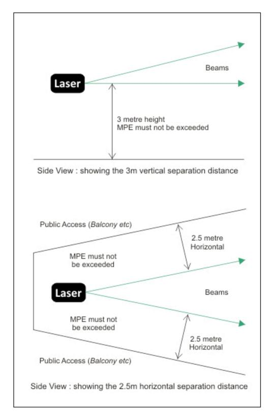
Note. The 3 metre height specified is not the height of the actual projector, but it refers to the height of the laser effect. Therefore having the laser projector positioned at 3m height and aimed directly down is not what the guidance is saying.
