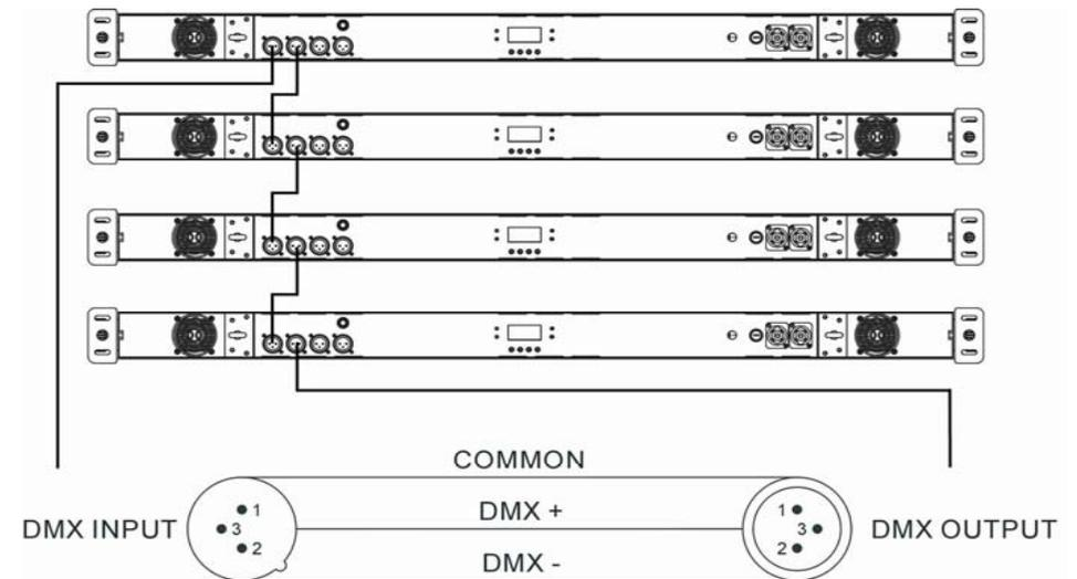
Termination reduces signal errors and avoids signal transmission problems and interference. It is always advisable to connect a DMX terminator. (Resistance 120 ohm 1/4W) between pin2(DMX-) and pin3(DMX+) of the last fixture.
