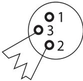
Termination reduces signal transmission problems and interference. it is always advisable to connect a DMX terminal, (resistance 120 Ohm 1/4 W) between pin 2 (DMX-) and pin 3 (DMX+) of the last fixture.
