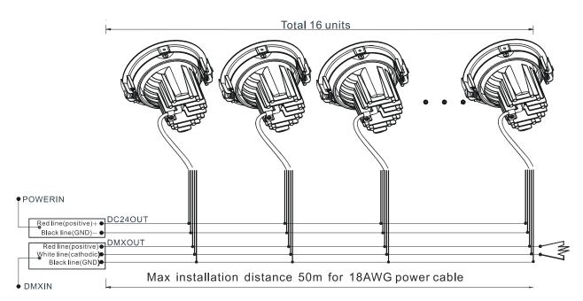
(Resistance 120 ohm 1/4W) between pin2(DMX-) and pin3(DMX+) of the last fixture. A 120 ohm 1/4Watt resistor must be added across the connections shown on the last fixture in the chain to eliminate corrupt DMX singals.
