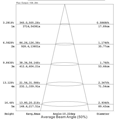
Note: the curves indicate the illuminated area and the average illumination when the luminaire is at distance.
