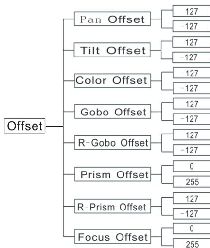
In the main functions, hold **Enter** button for at least 3 seconds into offset mode, use **DOWN** and **UP** button up to chose **Pan Offset**, **Tilt Offset**, **Color Offset**, **Gobo Offset**, **R-Gobo Offset**, **Prism Offset**, **R-Prism Offset** or **Focus Offset**, pressing **ENTER** Pressing **ENTER**
