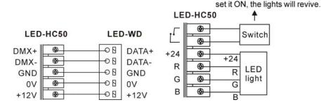
CAUTIONS : the LED controller total output power consumption is 50 watt.
