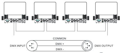
Termination reduces signal errors and avoids signal transmission problems and interference. It is always advisable to connect a DMX terminal. (Resistance 120 ohm 1/4W)between pin2(DMX-)and
