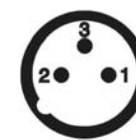
DMX - output XLR mounting-sockets (rear view):
