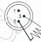
1. If you using a controller with 5 pins DMX output, you need to use a 5 to 3 pin adapter-cable.
