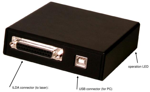
Pin 1 X+ Pin 2 Y+ Pin 3 blank/intensity + Pin 4 interlock Pin 5 red + Pin 6 green + Pin 7 blue + Pin 13 shutter Pin 14 X-Pin 15 Y-Pin 16 blank/intensity – Pin 17 interlock Pin 18 red -Pin 19 green -Pin 20 blue -Pin 25 ground
