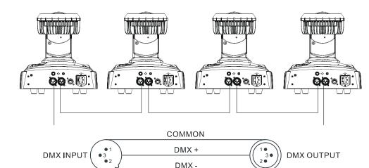
Termination reduces signal errors and avoids signal transmission problems and interference. It is always advisable to connect a DMX terminal.
