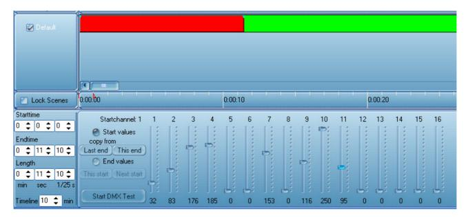
With the "Start DMX Test" button, you can see the output on your DMX device while adjusting the start- or end values.
