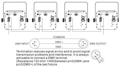
Connect the fixture together in a "daisy chain" by XLR plug cable from the output of the
