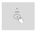
To return to normal mode, tap the Audio button a second time causing its LED goes out, the Audio mode is disengaged.
