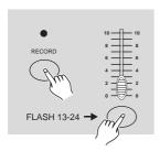
Press a Flash button between 13-24 while holding down the Record button. All LED will flash indicating the scenes have been programmed into memory.
