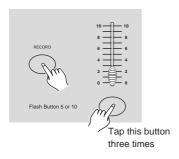
2. Tap the Flash button 5 or 10 three times while holding down the Record button.
