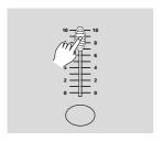
4. Move the desired Channel slider (13-24) to its maximum position to trigger the program, and the program will fade in depending upon current fade time.
