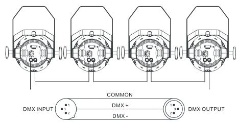
Termination reduces signal errors and avoids signal transmission problems and interference. It is always advisable to connect a DMX terminal.
