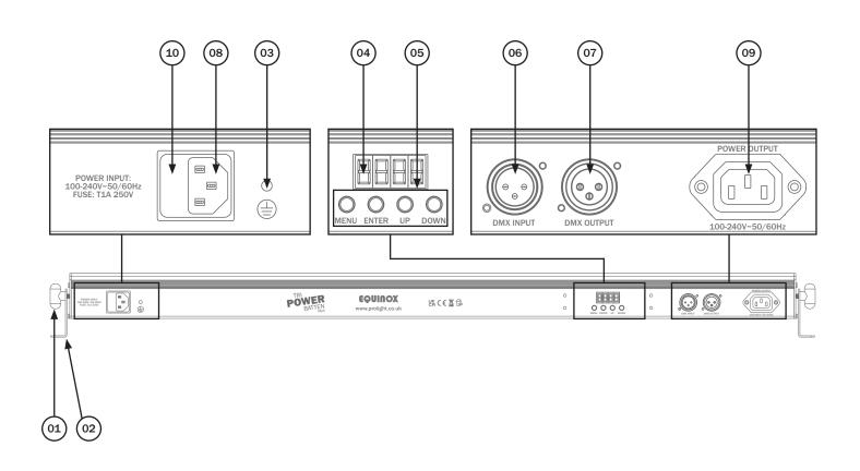
01 - Bracket tightening knobs
