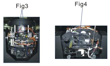
2. Follow the Fig.3 and Fig.4: Loosen the two screws and apart the entire assembly
